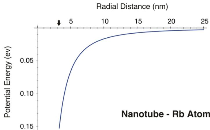
**Supplementary Figure 2. Attractive  $1/r^2$  potential for a neutral rubidium atom around a carbon nanotube charged to 150V.** The arrow indicates the surface of the 3.3 nm radius nanotube used in the experiments. The polarizability of Rb is  $47 \text{ \AA}^3$ .
